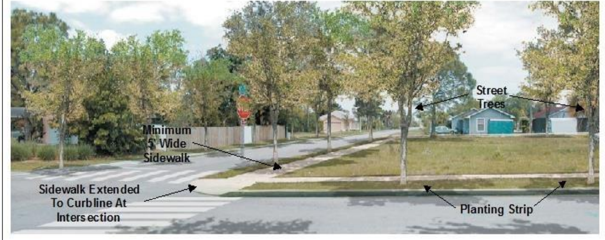
FIGURE 3: SIDEWALK DESIGN REQUIREMENTS
