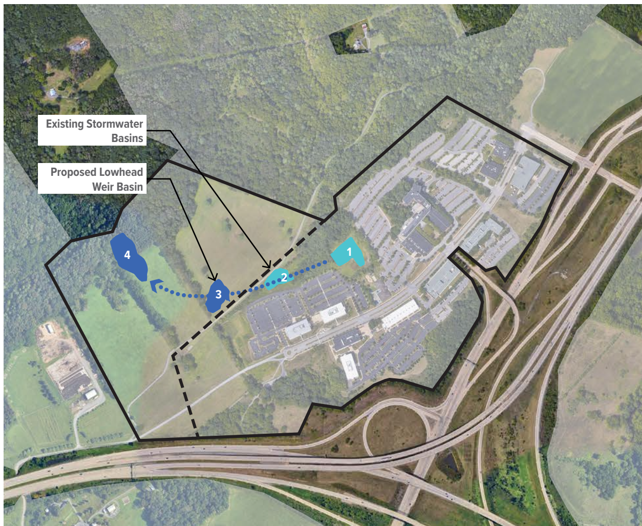
Figure 8: Layout of the approved 2012 stormwater plan for Innovation Park.
